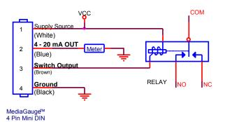
In the example shown above, the MediaGauge MG-MD is attached to an external power supply (Vcc), a current meter and a relay. The MG-MD has user programmable high and low pressure set points. We will assume the low set point has been set to 100 psi and the high set point has been set to 375 psi.
