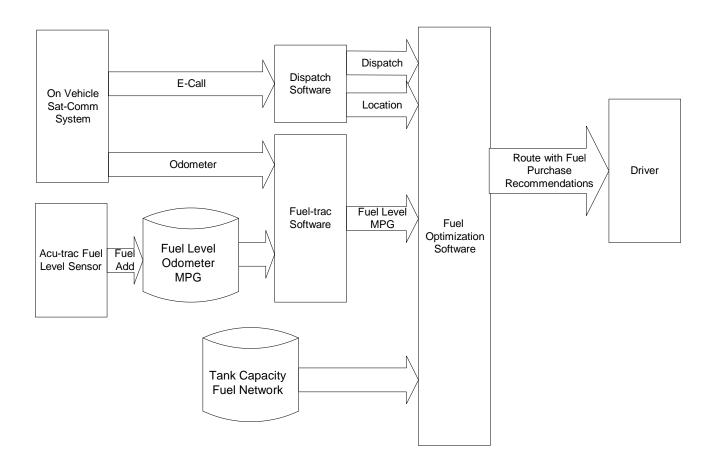
Figure 3. Fuel Optimization System with Acu-Trac<sup>™</sup> Fuel Level Sensor.
